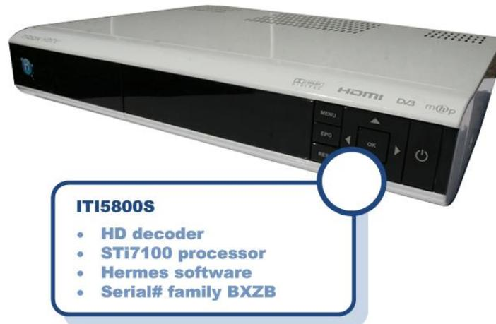
Fig. 3 ITI-5800S set-top-box-device.
